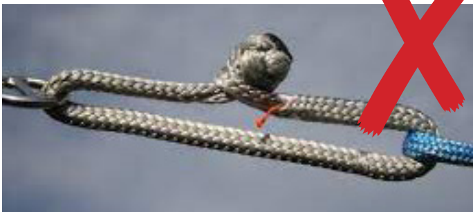
3. INCORRECT: NOT COMPLETELY TERRIBLE, BUT DEFINITELY NOT A BEST PRACTICE . THERE ARE A 'LOT' OF PEOPLE MAKING SOFT SHACKLES AND THE STYLE OF KNOT AND KNOT SIZE VARIES SIGNIFICANTLY. SMALLER OR POORLY CONSTRUCTED KNOTS, WHEN RIGGED IN THE CENTER LIKE THIS, CAN AND HAVE ALLOWED THE NOOSE TO SLIP OVER.
