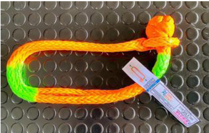
2. CORRECT: LOAD SHOULD BE WHERE THE GREEN MARKS ARE.
